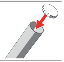
5 Place the tube in the barrel and close the launcher, see Section 3.2, step 5 and 6.
