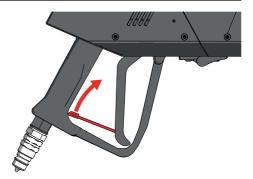
**3** Squeeze the handle to release the remaining pressure.
