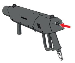
2 Remove the tube from the barrel.
