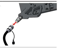
**6** Disconnect the  $CO_2$  hose from the  $CO_2$  Bottle to Hose Connector on the  $CO_2$  cylinder.
