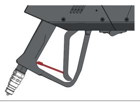
**2** Connect the  $CO_2$  hose to the  $CO_2$  quick connector.
