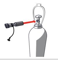
4 Connect the CO<sub>2</sub> hose to the CO<sub>2</sub> Bottle to Hose Connector on the CO<sub>2</sub> cylinder.
